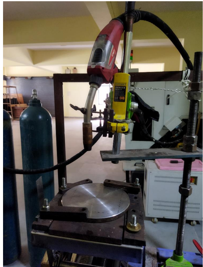
FIGURE I Experimental setup for cladding using CMT
