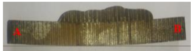
FIGURE VIII Distortion in the cut sample
