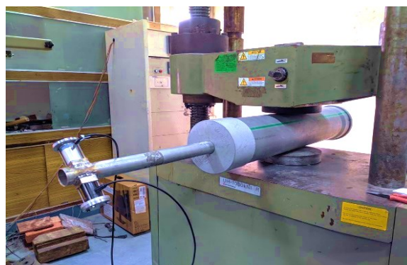
Fig. 3.-R6i & indigenous sensor connected with steel waveguide using silicone gel aid for acoustic transfer.
