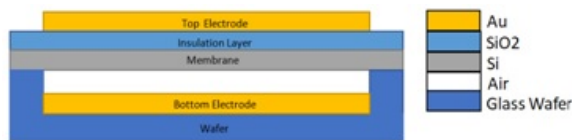
Fig. 3: Proposed CMUT cell structure
