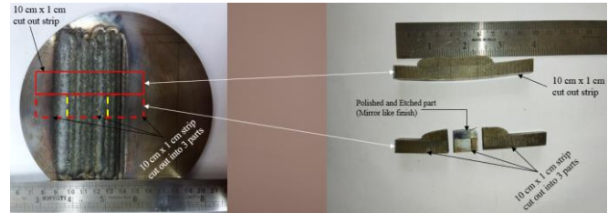
FIGURE VII High heat clad sample cutting
